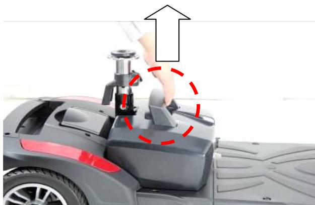
7. Pick up the battery pack and remove it from the scooter.
