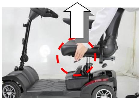
5. Push the Seat Rotate Lever while pulling up on the seat to remove.
